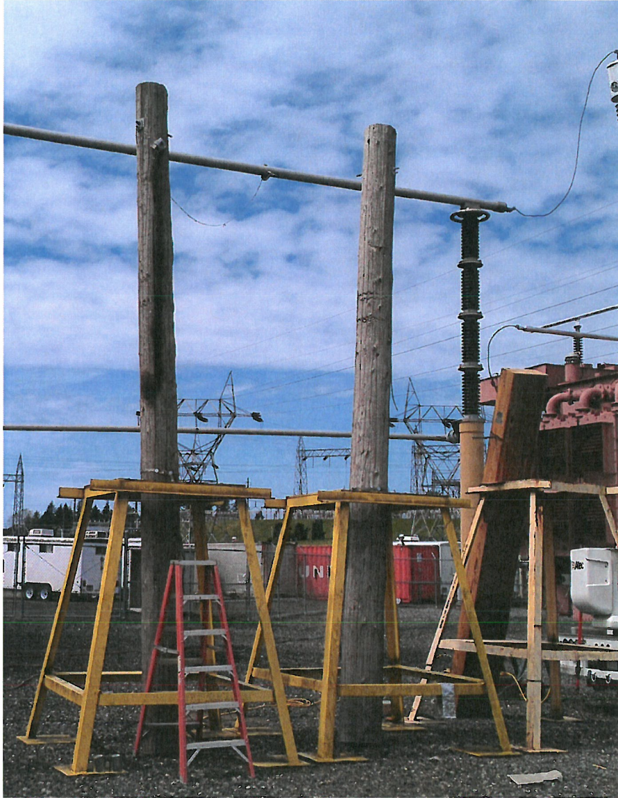
Figure 5 – Test Samples Erected Into Bushing Stands at the Fog Chamber.
