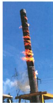
Figure 1 – Untreated Wood Pole Burning
