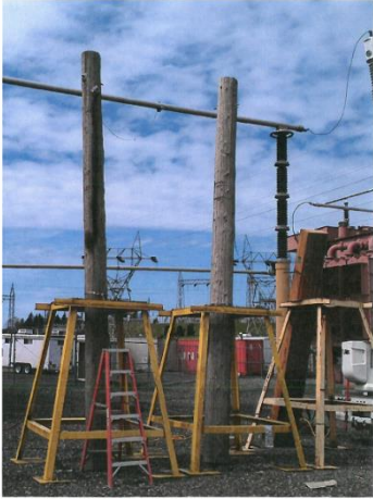
Figure 5 – Test Samples Erected Into Bushing Stands at the Fog Chamber.
